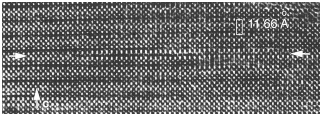
Fig. 10 The intercalation of fluorine into the Cu(1) layer occurring as an isolated defect (indicated by arrows); HREM image along [100]
